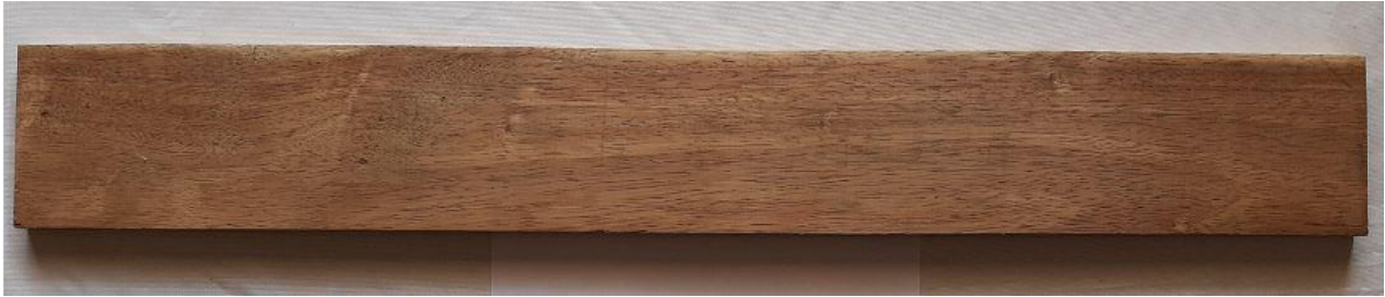
Figure 01. Planing (machining) property test sample of tetuya koroi wood
