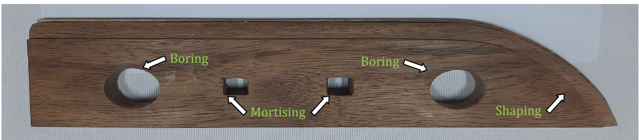
Figure 03. Shaping, boring and mortising (machining) test sample of tetuya koroi wood
