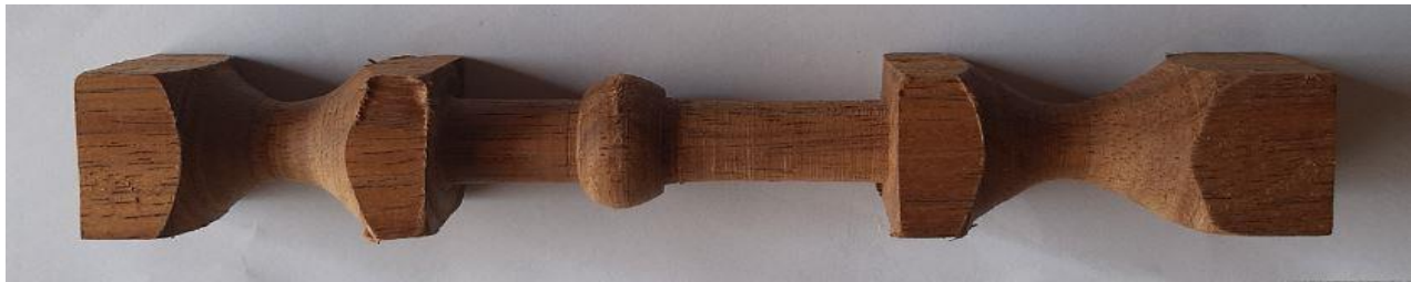
Figure 05. Turning (machining) property test sample of tetuya koroi wood
