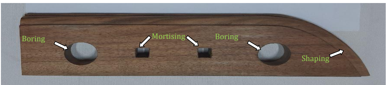
Figure 04. Shaping, boring and mortising (handtool) test sample of tetuya koroi wood
