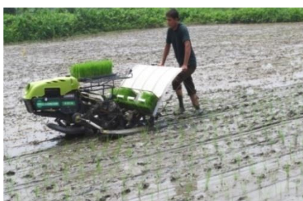
Figure 03. Transplanting operation performed by DP 480 and ARP-4UM rice transplanter.
