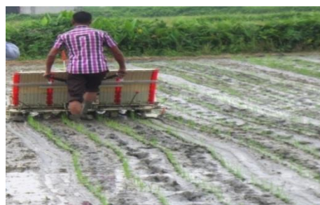
Figure 03. Transplanting operation performed by DP 480 and ARP-4UM rice transplanter.
