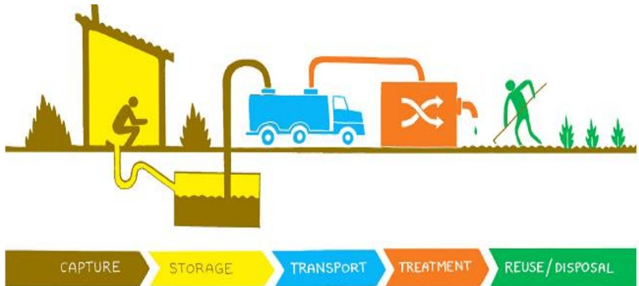
Figure 01. The key processes in a complete sanitation service chain.
