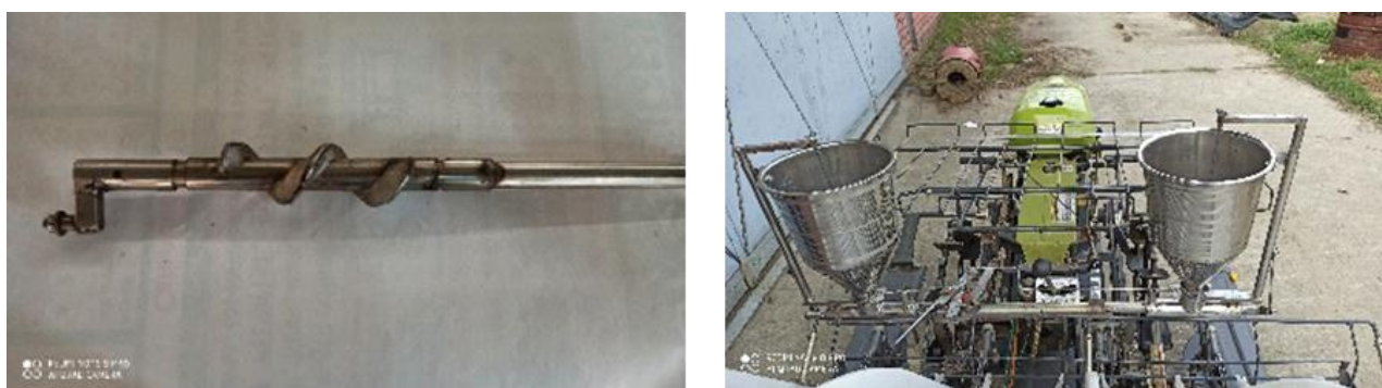
Figure 15. Spiral screw type metering device
