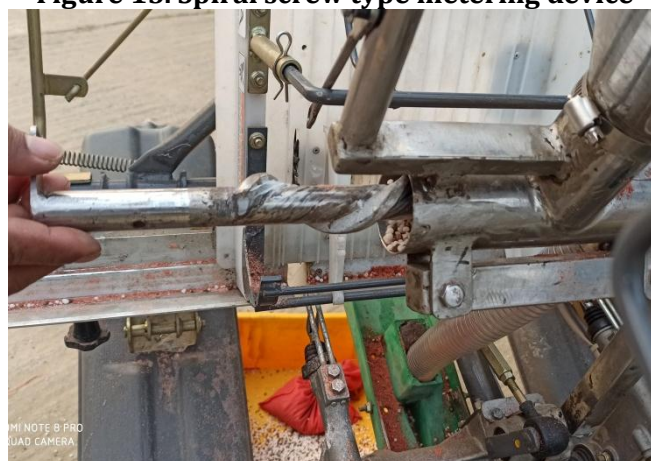
Figure 16. Spiral screw attached in the metering chamber
