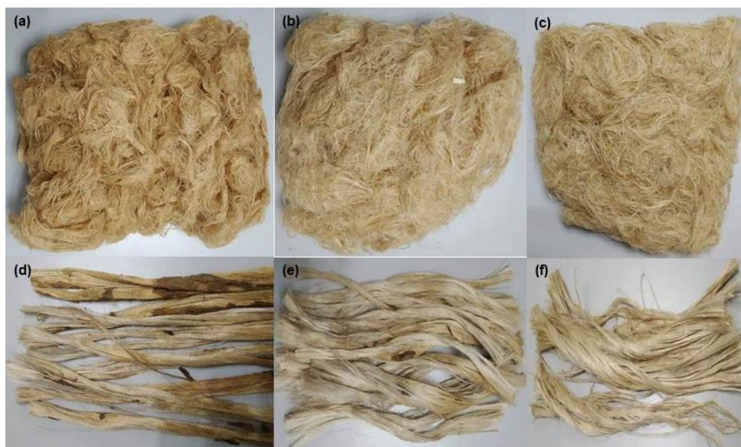
Figure 02. Image of machine extracted fibre and water retted fibre. a) Machine extracted fibre, bottom part; b) Machine extracted fibre, middle part; c) Machine extracted fibre, top part; d) Water retted fibre, bottom part; e) Water retted fibre, middle part; f) Water retted fibre, top part.
