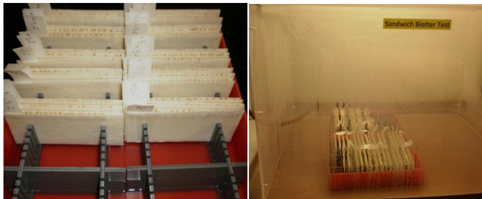
Figure 01. Sandwich blotter for rice germination test
